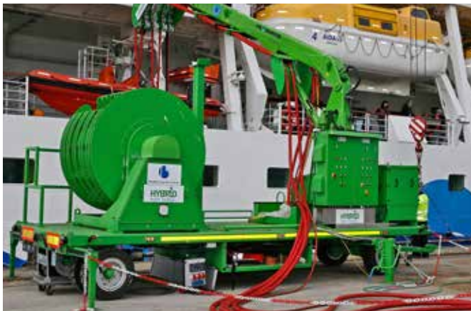
Energy supply of AIDAsol via the LNG hybrid barge
