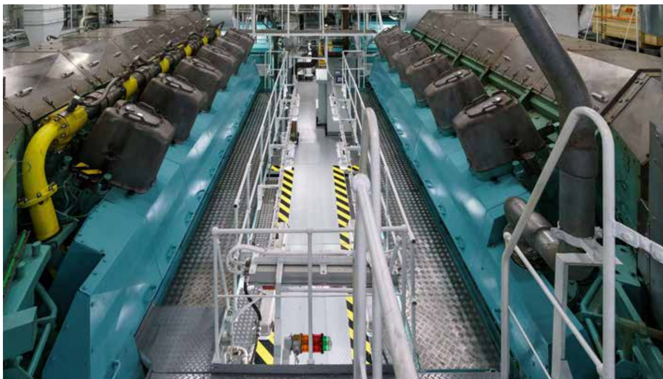
Dual-fuel engine onboard AIDAprima
