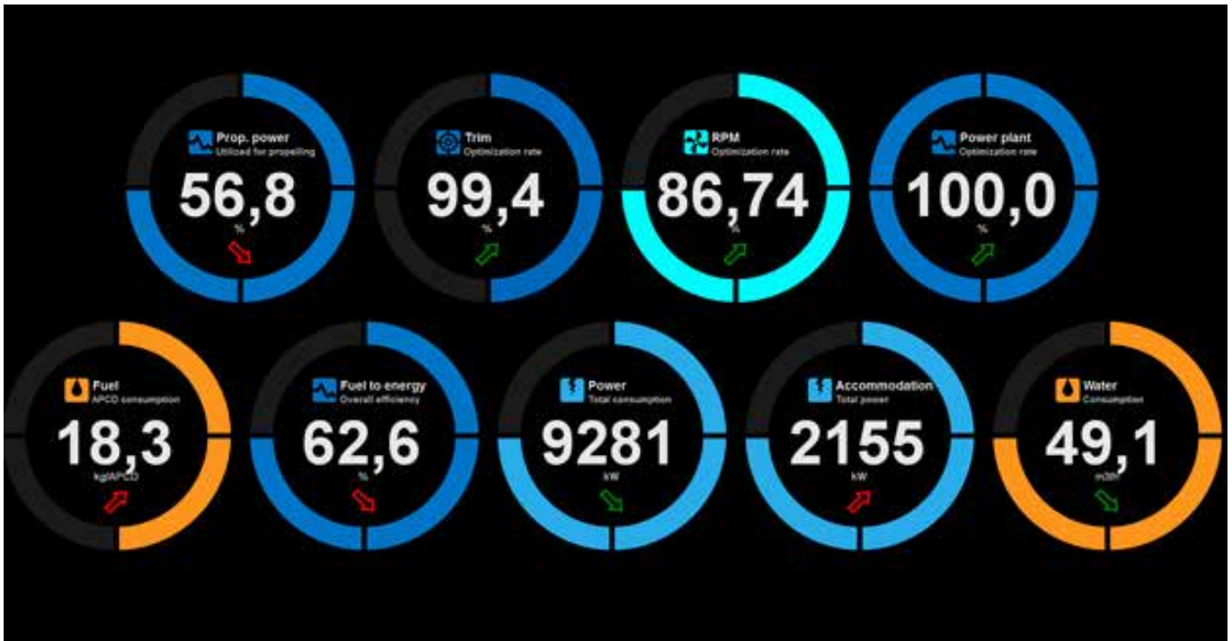
Energy monitoring and management system ABB EMMA
